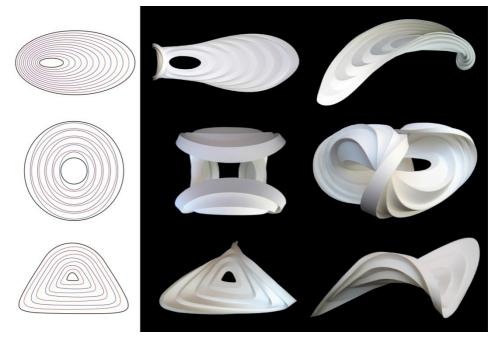
Figure 3: Variations of Bauhaus model by Duks Koschitz: ellipses with shifted foci, ellipses & circles, quadratic splines with 2 parabolas & 1 circle
