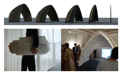
Figure 9: Tomohiro Tachi, Deployable Structure by assembly of curved foldings.
