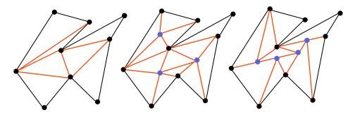
FIGURE 1. Types of triangulations: classic, proper, nonproper. Steiner points are blue.
