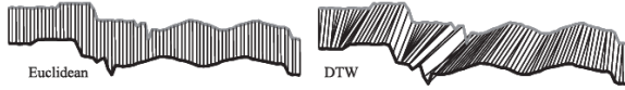
Figure 1: In Euclidean distance, the i th point of one time series is directly compared to the i th point of the other and is highly sensitive to alignment errors. LDTW accounts for misalignment by stretching and shrinking certain portions to provide the best match.
