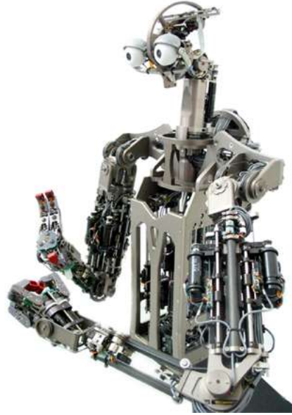
Figure 1: These experiments were conducted on the robot Domo. It has compliant, force sensing actuators in its arms and hands which allow it to safely explore its environment and its own body.
