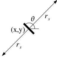
Fig. 4. This figure depicts the approximate locations in the image of the two votes at scale  $s$  cast by an edge with orientation  $\theta$  and position  $(x, y)$ .
