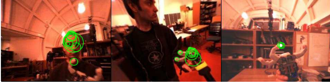
Figure 7-1: During human-robot interaction, hands, fingers, and faces are important perceptual features for visual attention. As shown in green, the InterestRegions module will often select these features because they are well modeled as rapidly moving convex edges.
