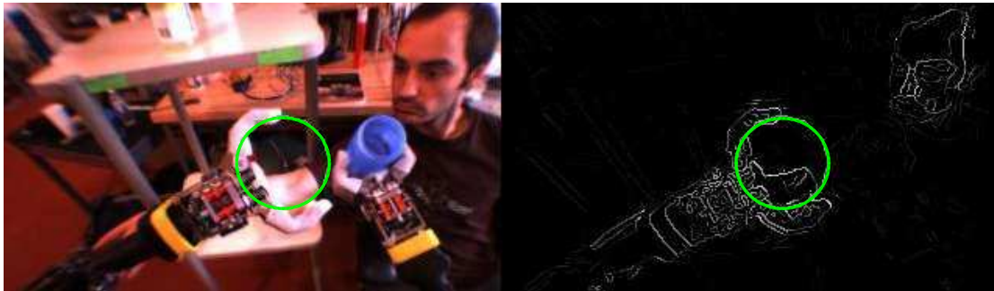
Figure 8-16: Left: The robot’s view during execution of PalmServo . This occurs in an everyday environment which includes a shelf, a person, as well as natural lighting and a cluttered background. The green circles mark the convex shape of the open hand which is being servoed. Right: The motion edges used in the detection of the palm.
