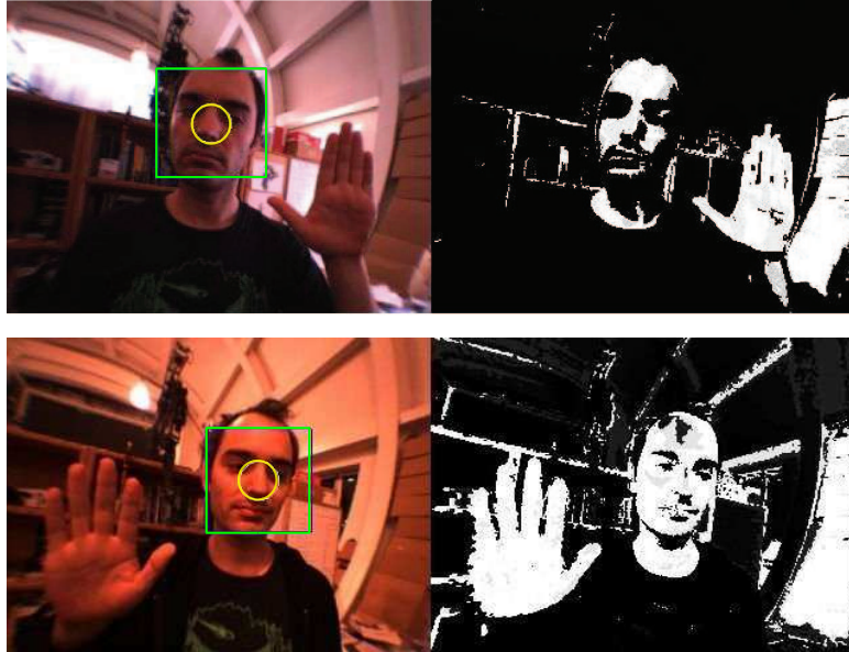
Figure 7-5: Output from the face tracker and skin color filter. The HSV skin color model adapts to the large shift in apparent skin hue between daylight (top) and night(bottom).
