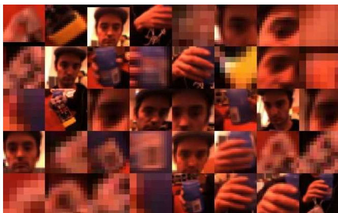
Figure 7-2: A random sample of image patches collected by the InterestRegions module. These predominantly contain hands, fingers, and faces.
