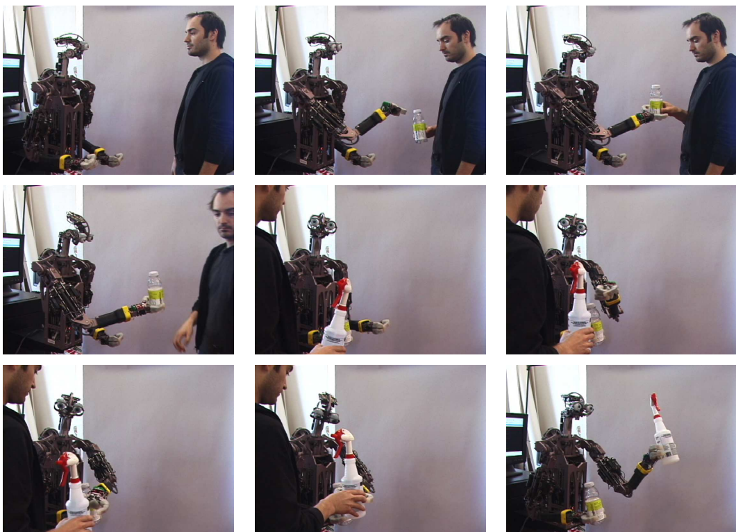
Figure 7-9: Domo executing the AssistedGrasp module to grasp a water bottle and spray bottle. Domo visually detects the collaborator and reaches towards him with an open hand. Domo detects the objects being placed in its hands and forms a power grasp on them.
