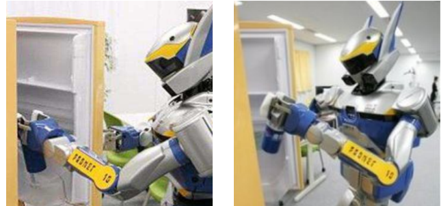
Fig. 1. Work with the AIST HRP-2 humanoid has combined high-level teleoperation with autonomous low-level perception and control. Here it is shown retrieving a drink from a refrigerator [1]. (Permission not yet acquired)
