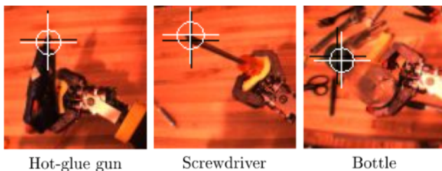
Fig. 4. Using visual motion and shape cues, Domo can detect the tips of tool-like objects it is rigidly grasping. The tip of a tool is a feature relevant to control of the tool. The white cross shows the kinematic prediction for the tool tip, based on noisy 2D detections, and the white circle shows the mean pixel error of the prediction relative to hand labels that were solely used for evaluation. The black cross marks the hand-labeled tip [4]
