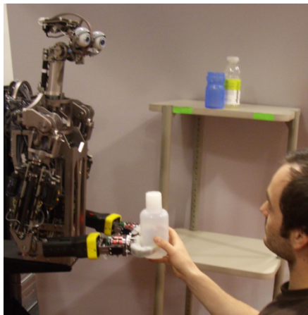
Fig. 3. The MIT CSAIL robot Domo works with a human to place cylindrical objects on a shelf [3].
