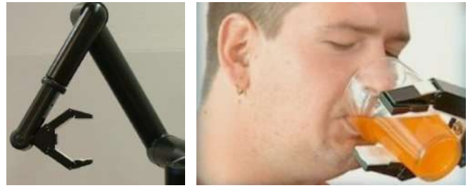
Fig. 2. The Manus ARM is designed to be attached to a wheelchair and has a joystick interface. It is controlled under close supervision by an operator. Researchers at UMass Lowell are expanding the autonomy of the arm in order to improve the assistance provided to the physically disabled. [1]. (Permission not yet acquired)
