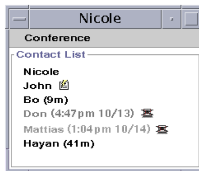
Figure 1. The Contact List provides awareness for a list of users by showing any computer input device idle time and any communication activity indicators for each user.
