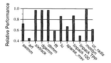
Figure 9. Slowdown due to disabling the stride-1 double-bandwidth mode.
