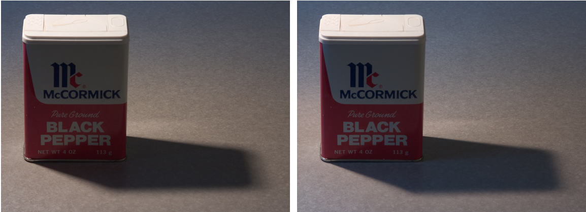
Figure 1-17: Photographs of shadows cast by square vs. triangular light sources. (Left) The box of pepper is lit by a square light source. (Right) The box is lit by a triangular light source. While the shadow penumbrae differ in shape, these differences are rather small.
