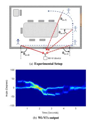
**Figure 3—Wi-Vi tracks a single person's motion.** (a) shows the experimental setup of a trial which consisted of a single person moving around in a conference room. (b) shows how Wi-Vi is able to track the motion of the person by computing the variation of the inverse angle of arrival with time, i.e.  $A'[\theta, n]$  for  $\theta$  in  $[-90^\circ, 90^\circ]$ .
