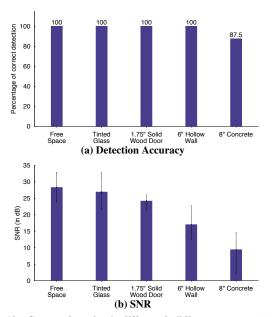
**Figure 12—Gesture detection in different building structures.** (a) plots the detection accuracy of Wi-Vi for different types of obstructions. (b) shows the average SNR of the experiments done through these different materials, with the error bars showing the minimum and maximum achieved SNRs across the trials.
