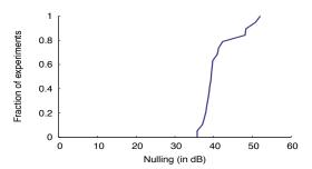
Figure 13—CDF of achieved nulling. The figure plots the CDF which shows the ability of nulling to reduce the power received along static paths.
