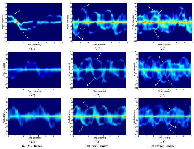
**Figure 8**—**Tracking human motion with Wi-Vi.** The figures show output traces with a different number of humans after processing with the smoothed MUSIC algorithm. They plot  $A'[\theta, n]$  where  $\theta$  is the angle in [-90, 90] is plotted on the y-axis and time is on the x-axis. (a) shows traces for one human; (b) for two humans; and (c) for three humans moving behind the wall of a closed room.
