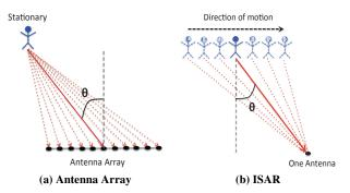
Figure 1—A Moving Object as an Antenna Array. In (a), an antenna array is able to locate an object by steering its beam spatially. In (b), the moving object itself emulates an antenna array; hence, it acts as an inverse synthetic aperture. Wi-Vi leverages this principle in order to beamform the received signal in time (rather than in space) and locate the moving object.
