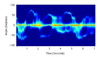
Figure 4—Wi-Vi tracks the motion of two humans. The figure shows how the presence of two humans translates into two curved lines whose angles vary in time, and one straight line which corresponds to the DC.
