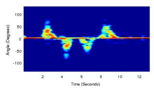
Figure 5—Gestures as detected by Wi-Vi. The figure shows a sequence of four steps: step forward, step backward, step backward, step forward. Forward steps appear as triangles above the zero line; backward steps appear as inverted triangles below the zero line. Each pair of steps represents a gesture/bit: the first two represent bit '0', the second two represent bit '1'.
