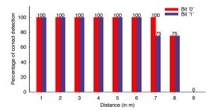
**Figure 10—Accuracy of Gesture Decoding as a Function of Distance.** The figure shows the fraction of experiments in which Wi-Vi correctly decoded the bit associated with the performed gesture at different distances separating the subject from the wall. Note that Wi-Vi decodes a gesture only when its SNR is greater than 3dB; this explains the sharp cutoff between 8 and 9 meters.
