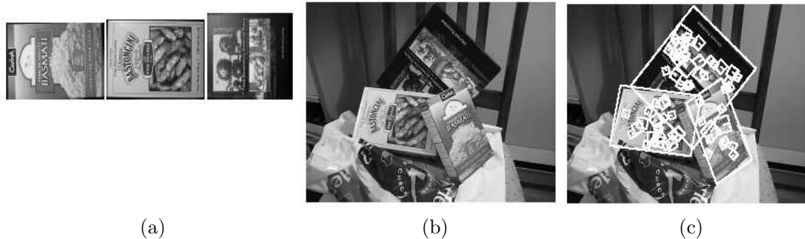
Figure 2.3: The object recognition system of Lowe. (a) Objects stored in the system. (b) Query image. (c) Image with object superimposed. The small rectangles are the features matched to the object models.
