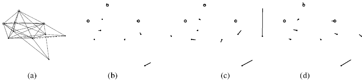
Fig. 5. (a) Small (ten-sensor) graph and the observable pairwise distances; calibration is performed relative to the location of the sensors shown in green. One distance (shown as dashed) is highly erroneous, due to a measurement outlier. (b) The MAP estimate of location, discarding the erroneous measurement. (c) A nonlinear least-squares estimate of location is highly distorted by the outlier. (d) NBP is robust to the error by inclusion of a measurement outlier process in the model.
