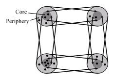
**Fig. 1.** A simulated 2-dimensional hypercube with four nodes, each consisting of a core and a periphery. All peers within the same node are completely connected to each other, and additionally, all peers of a node are connected to all core peers of the neighboring nodes. Only the core peers store data items, while the peripheral peers may move between the nodes to balance biased adversarial changes.
