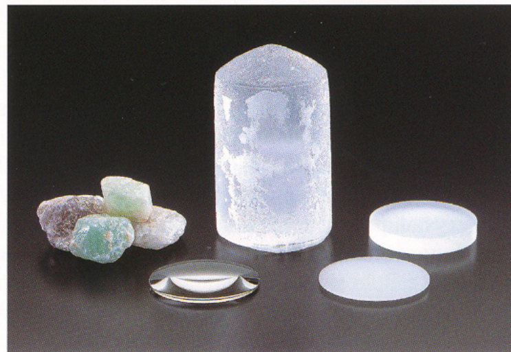
Photo-12 Artificial Fluorite Crystals and Fluorite Lenses
