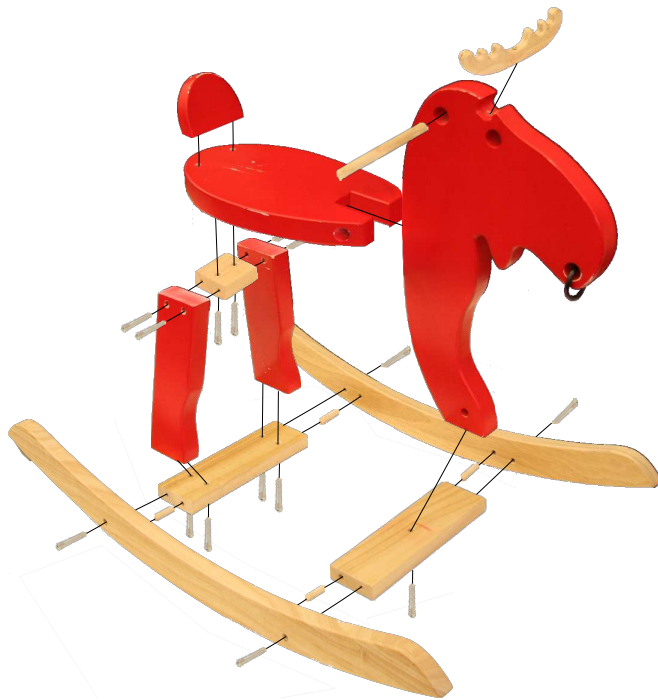
Fig. 1: We describe a decentralized parallelizing assembly planner for structures such as the IKEA Ekorre rocking moose. Its assembly can be parallelized into as many as five parallel tasks.
