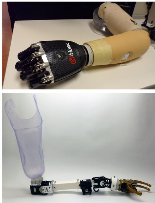
Fig. 1. Augmentative and restorative prosthetics are of specific interest for incrementally integrating AI into a robotic setting. *Top*: commercial limb system prescribed to an amputee for use during daily life. *Bottom*: research robot limb system with direct access to a rich sensorimotor stream [4].
