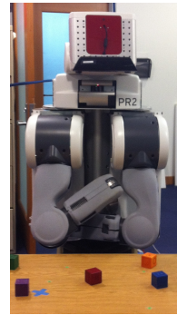
Figure 1: A robot considers a blocks-world problem. At the swampy (low) level it must process high-dimensional visual and laser data, and actuate its joints such that it can pick up and move blocks without colliding with itself or the table. At the crispy (high) level, it can make abstract plans about the placement of blocks on top of each other, without considering the details of movement or perception.
