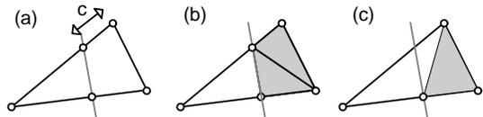
Figure 4. A triangle element intersected by a cutting plane (a). If  $c > \rho$ , both intersection points are added to the mesh (b). Otherwise the top point is not added to the mesh (c). The cut is formed by separating the two regions above (white) and below (gray) the plane.
