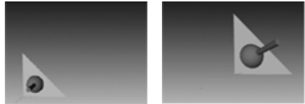
Figure 1. Two frames showing the positioning a simple object (triangle) by grabbing it with the haptic device (stick and sphere).
