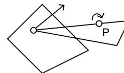
Figure 2. The Phantom pointer (P) is positioning a triangular object that intersects another object. The user feels a force that opposes the penetration (straight arrow), and also a torque (curved arrow).
