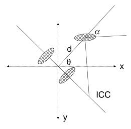
Figure 2. Bicycle/tricycle kinematics. The shaded ovals represent the three wheels of *Trike*. The instantaneous centre of curvature (ICC) must lie at the intersection of lines orthogonal to, and passing through the rotation axis of each wheel.
