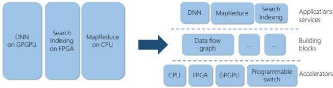
Fig. 3. Programming abstractions: from a vertical to a horizontally integrated stack. Examples are taken from [10], [22], [35].
