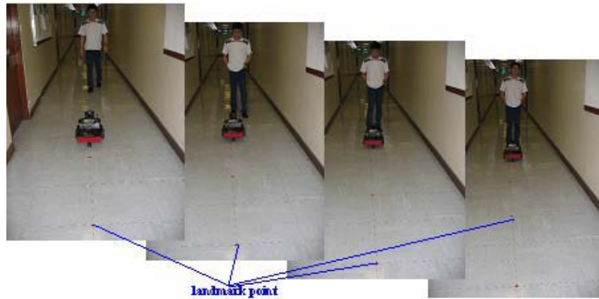
Figure 5: Pioneer 1 mobile robot map building in a dynamic corridor environment at HKPU
