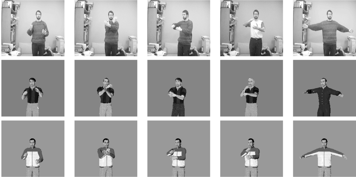
Figure 4-4: Examples of upper body pose estimation (Section 4.4). Top row: input images. Middle row: top matches with LSH on the SSC embedding. Bottom row: robust constant LWR estimate based on 12 NN. Note that the images in the bottom row are not in the training database - these are rendered only to illustrate the pose estimate obtained by LWR.
