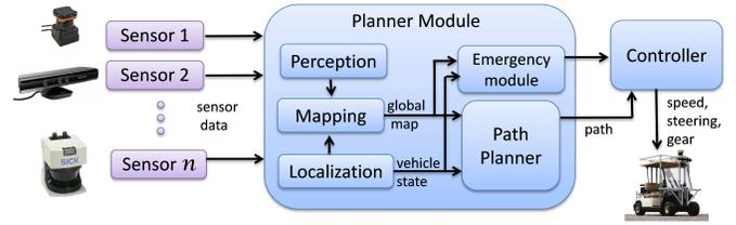
**Figure 3—High-level Architecture of Autonomous Vehicles** Sensor information from various sensors is provided to the path planner module which computes a path for the vehicle to navigate along.
