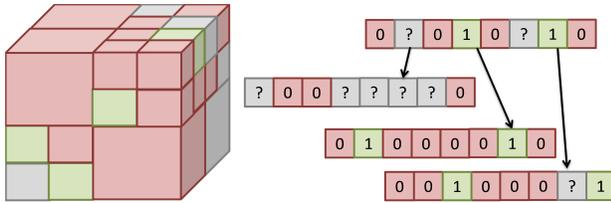
**Figure 5—Octree Representation** Representation of 3D-point cloud using a 2-level Octree. Vertices that are unoccupied are not expanded; vertices that are completely occupied or unknown are terminated by special leaf vertices; these have been omitted for clarity.
