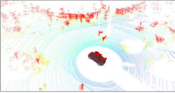
**Figure 2—An example of sensory information gathered during autonomous driving.** The figure shows a 3D-point cloud of a road obtained using a Velodyne laser sensor. The colors refer to elevation from the ground. A 3D-point cloud is a set of  $(x, y, z)$  coordinates of points lying on the surface of obstacles.
