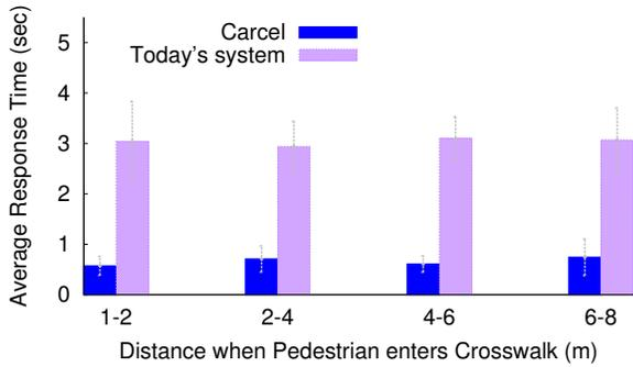
**Figure 7—Time Delay Averages for Carcel and baseline.** Distances on the x-axis are grouped into bins of two meters representing distances of the golf car from the crosswalk at the time the pedestrian enters the crosswalk.
