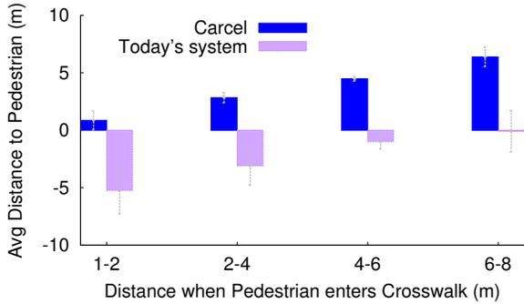
**Figure 8—Comparison of golf car distance from the crosswalk when the pedestrian enters the crosswalk to the distance from crosswalk at which the receiver issues a stop command to the vehicle.** Distances on the x-axis are grouped into bins of 2 m.
