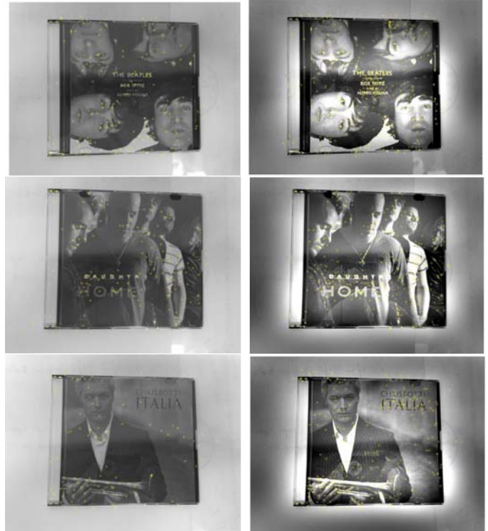
Fig. 11. Dull images (L) offer more features when dynamic range is stretched (R)
