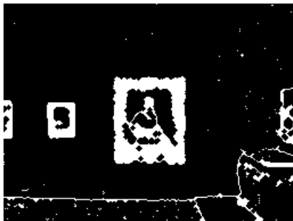
Fig. 8. Morphological closing of the Sobel edge map with a radius-one diamond structuring element. Lines are bridged, but not all holes are closed.
