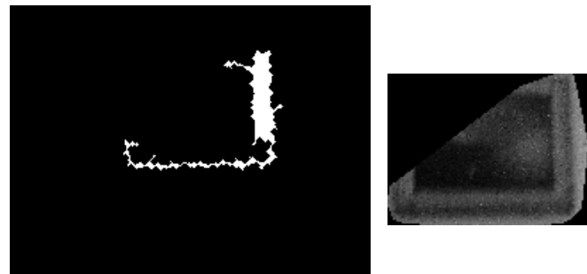
Fig. 13. Example of failed region segmentation due to over-thresholding. The triangular shape (and therefore proportion of the bounding box) of the resulting region raises the flag, leading to a lowered threshold in the next trial.
