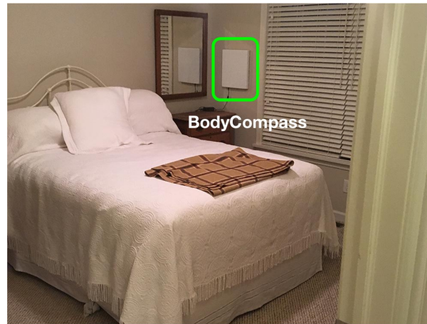
Fig. 1. BodyCompass in one of our deployments. The white box mounted on the wall is the radio. It uploads the RF signals to the cloud where the model processes them to extract sleep posture.
