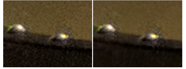
Figure 8: Spatial denoising failing to suppress noise around strong high contrast features. Note the spatial denoising is effective throughout the image, except near the strong specular highlights on the metallic rivets.
