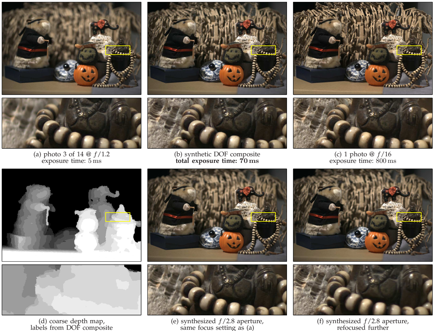
Fig. 7. HAMSTER dataset. Light efficient photography timings and synthesis, for several real scenes, captured using a compact digital camera and a digital SLR. (a) Sample wide-aperture photo from the synthetic DOF sequence. (b) DOF composites synthesized from this sequence. (c) Narrow-aperture photos spanning an equivalent DOF, but with much longer exposure time. (d) Coarse depth map, computed from the labeling we used to compute (b). (e) Synthetically changing aperture size, focused at the same setting as (a). (f) Synthetically changing focus setting as well, for the same synthetic aperture as (e).
