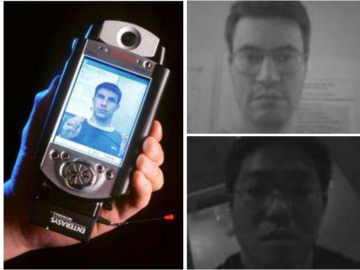
Fig. 2. The iPAQ handheld computer used in our study, along with two sample images collected in the iPAQ.
