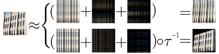
Figure 6. Approximation of a facade image with the top three singular components  $\sum_{i=1}^3 \sigma_i \mathbf{u}_i \mathbf{v}_i^T$ . **Top:** SVD of the original image. **Bottom:** SVD of the rectified image by TILT.
