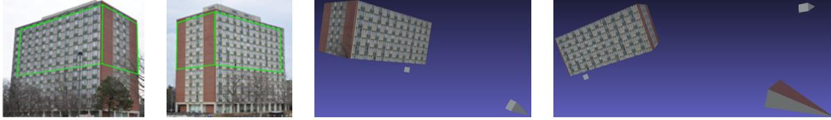
Figure 1. **Left Pair:** Example of matched facades of a building. **Right Pair:** Automatically reconstructed 3D model from *only four uncalibrated* images around the building by our method. Each image covers a pair of facades. The pyramids show the estimated location of cameras.
