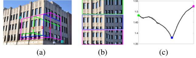
Figure 3. Identifying the intersection line  $l$  of two facades. (a) Three different intersection hypotheses for the two adjacent 4-sided polygons. (b) The unfolded joint textures: each corresponds to one of the hypotheses shown in (b), as indicated by the color of its boundary. (c) The value of (3) as a function of the location of the intersection line. It is minimized precisely at the correct location (the blue line).
