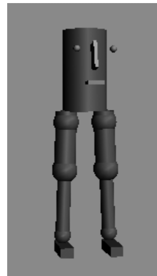
Fig. 1. The humanoid model is shown having the basic structural features necessary to simulate human standing in three dimensions, including legs with hip, knee and ankle.
