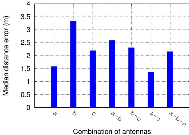
Fig. 5: Effect of different combinations of receiver antennas ( $a, b, c$ ).
