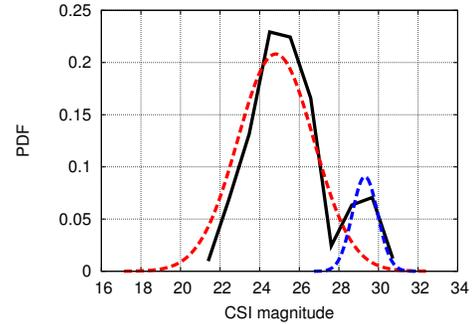
(a) PDF of the CSI magnitude showing the Gaussian mixture representing the two clusters.
