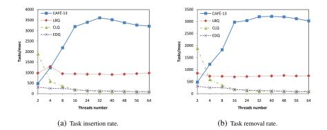
**Fig. 2.** Task insertion and retrieval rates (equal numbers of producers and consumers). The throughput of CAFÉ-13 increases up to 32 threads (the number of hardware threads in the system). In this configuration it is  $\times 30$  faster than the Michael-Scott ConcurrentLinkedQueue and over three times higher than all other implementations, including the ones not providing FIFO. CAFÉ continues demonstrating high throughput even when the number of threads increases up to 64.
