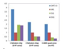
Fig. 3. Throughput on different hardware architectures, normalized by the throughput of LBQ. There are 6 producer threads and 6 consumer threads.
