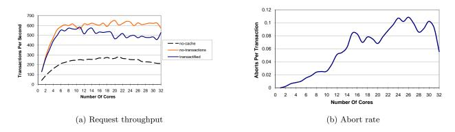
Figure 8: Medium locality workload (s = 1), Apache in single-process mode. The abort rate increases with the number of cores, which explains the decline in the transaction rate.
