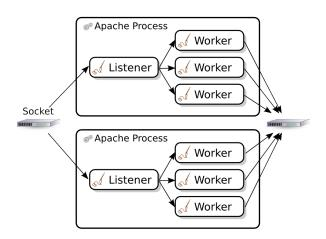
Figure 1: Apache worker MPM architecture.
