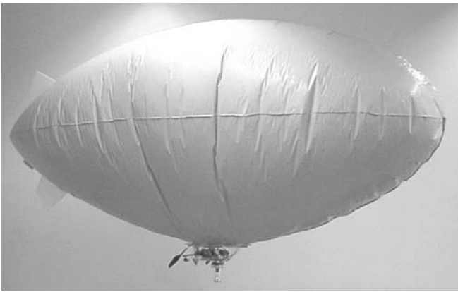
Figure 7. The autonomous flying robot, Melissa. Left: Melissa consists of a helium balloon, a gondola hosting the onboard electronics, and a host computer. The balloon is 2.3m long and has a lift capacity of approximately 400g. Right: Inside the gondola, there are 3 motors, a four-channel radio transmitter, a miniature panoramic vision system and image transmitter, and the battery.
