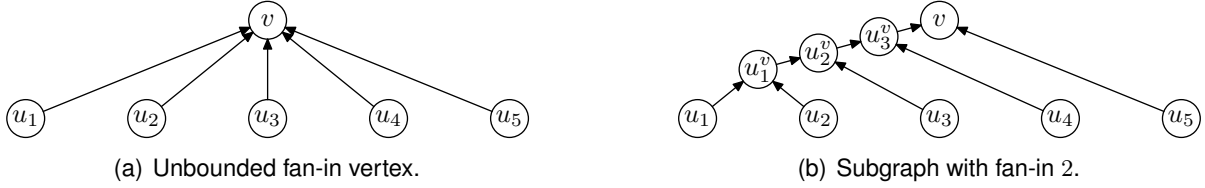
Figure 14: Conversion of unbounded indegree DAG to indegree 2 DAG.
