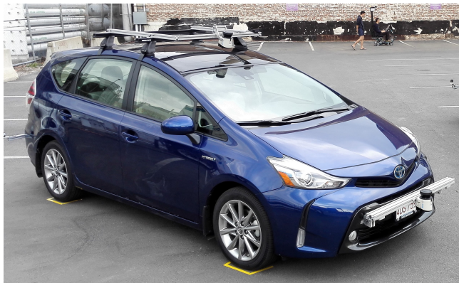
Fig. 1. The converted Toyota 2015 Prius V, a parallel autonomy research platform. The car is outfitted with sensors to enable fully autonomous driving, a drive-by-wire conversion and low-level controllers which are designed to fuse the desired input from the human with the autonomy software control output to provide safe acceleration and speed.
