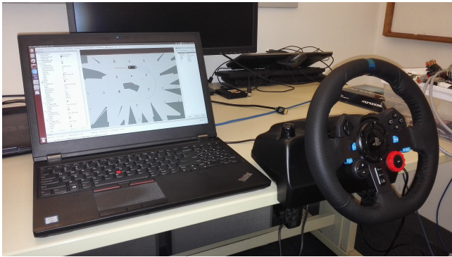
Fig. 9. A steering wheel and pedals (not shown) are interfaced to provide a standard and uniform user interface to test parallel autonomy with human inputs in Drake.
