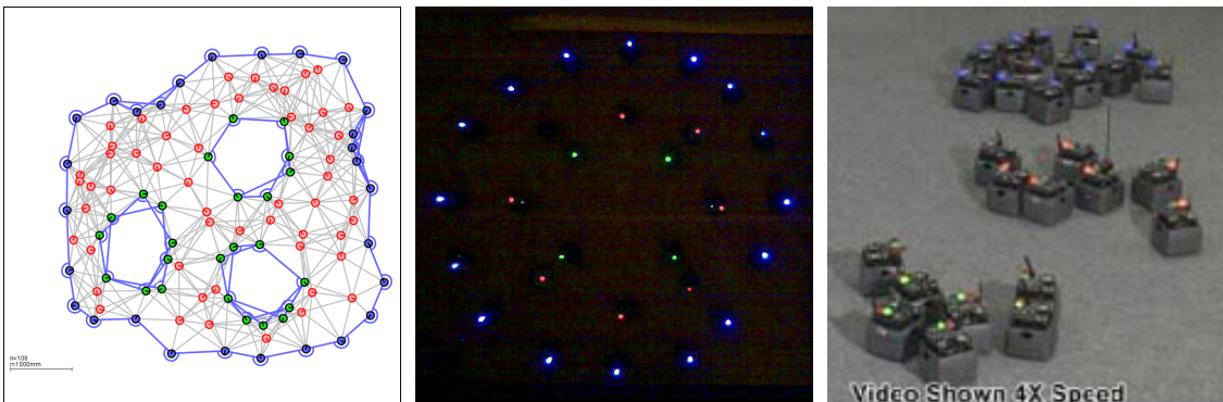
(d) Boundary detection and sub-graph construction (e) Robots detecting the external boundary (blue) and an internal assignment void (green) (f) Robots executing dynamic task assignment
