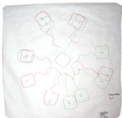
Figure 28: Left: The avoidRobot behavior produces the traces shown. The red robots were started facing upper-left, and the green traces are from robots released facing the upper-right. The summation of orientToRobot and moveForward produces the “J”-shaped traces shown. Right: The data shows path efficiency declines as the rotation angle increases. Average path efficiency is 69%, and average distance accuracy is 93%.
