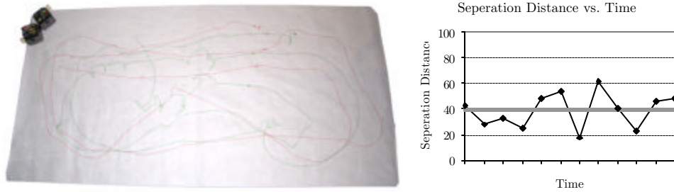
Figure 27: Left: The followRobot behavior produces the traces above. The red robot is the leader, and the green the follower. Each robot is programmed to “twitch” every two seconds so that their separation distances can be compared from the traces. Right: The commanded distance is 40 cm, and the average measured inter-robot separation is 39 cm, which yields a accuracy of 97% and a path efficiency of 114%. Both of these metrics were distorted somewhat because turns allow the follower to take “shortcuts” and round the corners on a shorter path than the leader.
