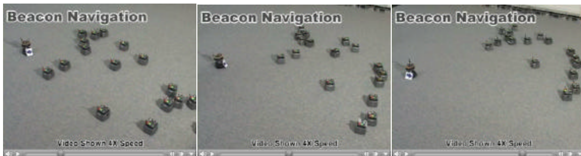
Figure 24: The pictures above show how a long-range ISIS beacon can be used with the matchHeadingToRobot behavior to guide the robots in along global heading. The robots are trying to move “north”. As the beacon is rotated, all the robots change their direction accordingly. If the heading of the beacon is kept constant, the robots can use it like a compass to determine their absolute heading. Multiple beacons can be used to cover the entire workspace.
