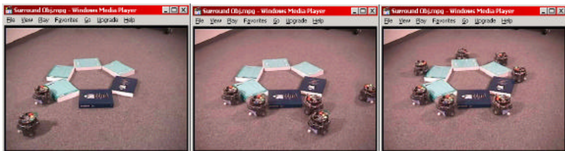
Figure 63: The surround demo guides a group of robots to autonomously surround an object.
