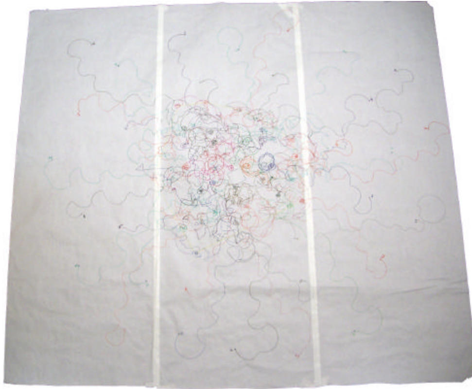
Figure 57: These traces show results of the clusterOnSource behavior. The outline of the source robot is located in the center of the densely marked section.
