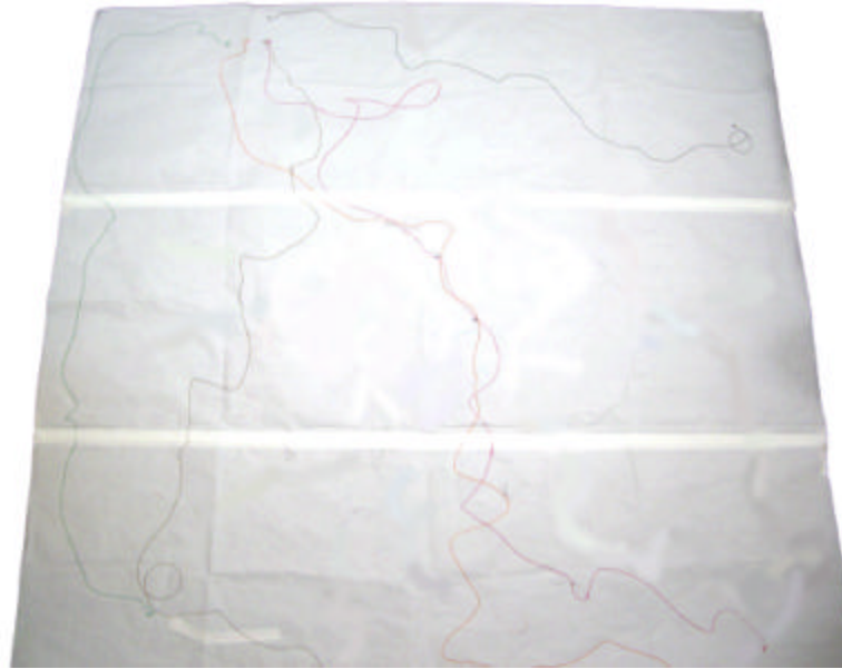
Figure 54: These traces show the results of the navigateGradient behavior from different starting locations. This behavior produced an average path efficiency of 28%.
