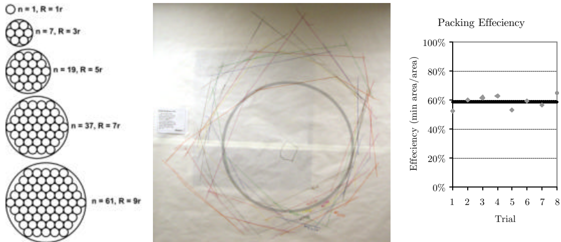
Figure 59: Packing efficiency is defined at minimum area / used area. Right: Optimal packing efficiency is achieved when robots form a tightly packed hexagonal pattern. Middle: The convex hulls formed by the clustering algorithm are shown as different colored outlines, and an optimal circle of radius R is shown in gray. Left: The average packing efficiency of the clusterOnSource behavior was 59%.
