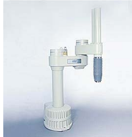
Figure 1-4 Adept Direct-Drive robot
