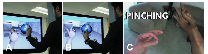
Figure 3: Illustration of potential Digits application scenarios. A+B) Continuous interaction with 3D content on a large display. C) Gesture recognition performed on reconstructed hand model.
