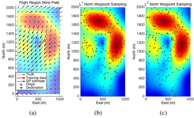
Fig. 1: (a) True and estimated 2D wind field across the flight region. The gradient of the estimated wind field is given by the underlying surface plot. A set of 200 random waypoint samples drawn from the (b)  $L^1$  norm and (c)  $L^2$  norm gradient distributions. Samples are shown as circles.
