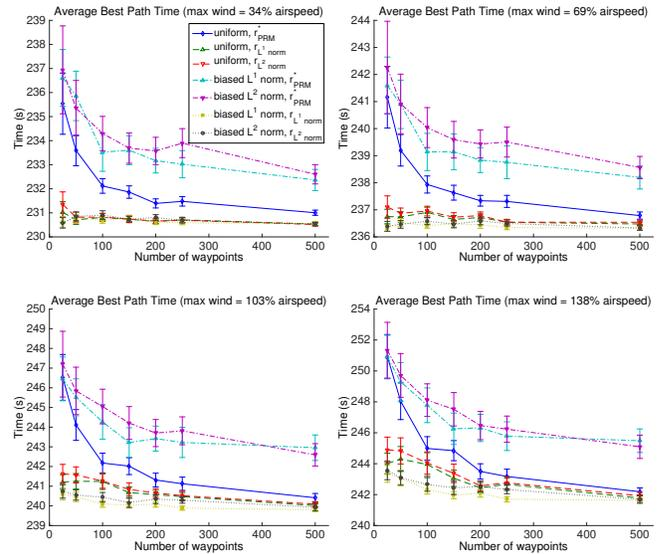
Fig. 2: Fastest time to travel from the origin node to the destination node across the four tested wind fields averaged over 100 random waypoint generations. 7 PRMs were tested, using either uniform or biased random sampling to select waypoints, and either a constant connection radius, defined as the lower bound of the PRM\* radius in (1), or a variable connection radius, computed from (4), to connect the waypoints in the graph.
