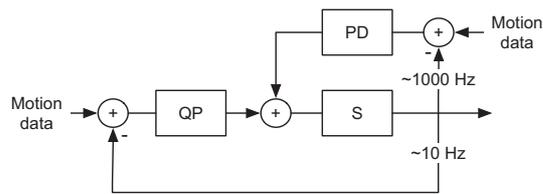
**Figure 1:** An overview of McSim’s design. At 40 to 100 Hz, the predictive model solves a quadratic program for the joint and external forces that track the reference motion. These forces are adjusted by a low gain proportional derivative component that computes feedback forces at every simulation time step (1-10kHz). Our controller can work with any black-box simulator.
