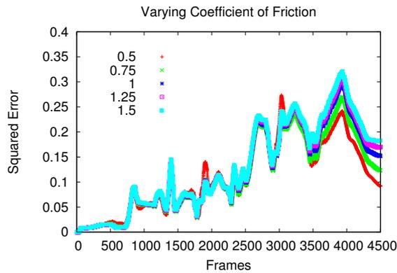
**Figure 5:** In these plots, the squared error is shown for a walking motion where the coefficient of friction in the predictive component is varied from 0.5 to 1.5. The simulator's coefficient of friction was fixed at 1. For walking motions, the error is not greatly effected by the coefficient of friction used in the model. When the predictive model's coefficient of friction exceeds the actual coefficient of friction, performance is worse, but only slightly.
