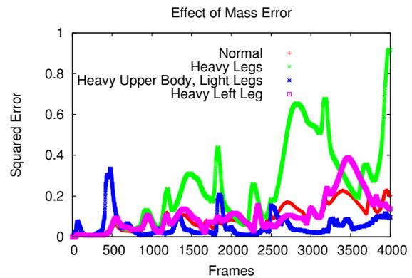
**Figure 4:** Shown are plots of squared error over time for four versions of the 2D model tracking the walking motion. The modifications are described in the legend. McSim is more sensitive to errors in the mass properties of the legs.
