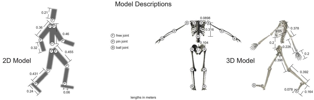
**Figure 7:** The models. A free joint has six degrees of freedom and is represented by a position and a quaternion. A pin joint has one degree of freedom and is represented by an angle of rotation. The center of mass of each link is located at the center of the link. Inertial and joint stiffness properties are listed in Table 2 and 3.
