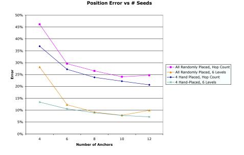
Fig. 5. Graph of position error versus number of seeds for two different seed placement strategies. Position error for smoothed hop count and 6 level radio strength distance estimates are shown.
