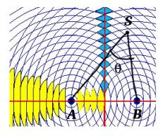
Fig. 4. Error in position relative to two seeds can be approximated as a parallelogram. The area of this parallelogram depends on the angle  $\theta$ . When  $\theta$  is 90 degrees the error is minimized, however in certain regions  $\theta$  is very small resulting in very large error.
