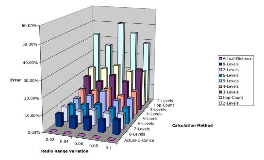
**Fig. 7.** Graph of the effect of 0-10% communication radius variation and different levels of signal strength quantization on location estimation accuracy.
