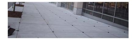
Fig. 9. Motes placed on a 5x7 grid aligned with an outside cement sidewalk.
