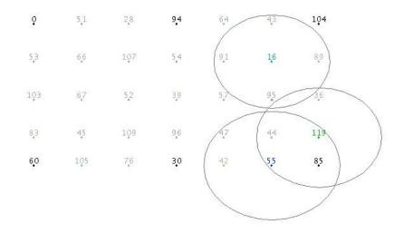
Fig. 10. Ranging information for node 95. Node 95 has ranging information for nodes 55, 119, and 16.
