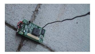
Fig. 8. A Berkeley MICA2 mote with sensor board.
