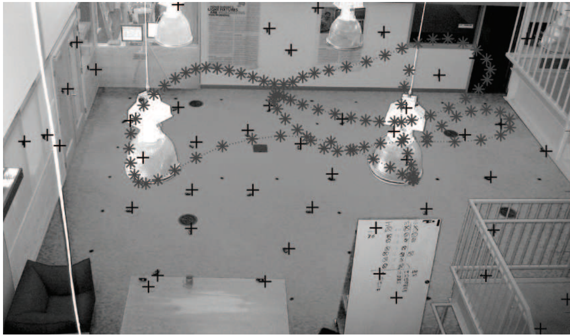
Figure 6-16: Results for the 55 node 3D experiment. Estimated positions are plotted with crosses, and a portion of the recovered mobile trajectory is plotted using asterisks and a dotted line. LaSLAT localized this network with a mean error of 7 centimeters.
