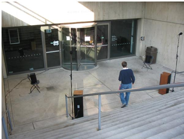
Interactive Sound Installation (Computer, 8-Channel Soundcard, 8 Loudspeakers, 2 Stereo Microphones, Max/MSP)
