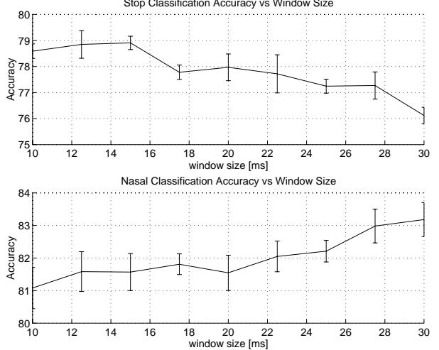
**Figure 2:** Comparison of within-class stop and nasal classification as a function of Hamming window duration. The vertical bars show one standard deviation in the performance calculated over five trials of mixture model training.
