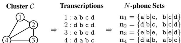
**Fig. 3.** Conversion of cluster nodes into groups of  $n$ -phones. The intervals under the nodes are phonetically transcribed, then separated into sets of  $n$ -phone sequences. In this example,  $n = 3$ .
