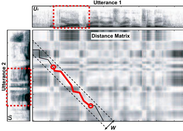
**Fig. 1.** The segmental DTW algorithm. As in normal DTW, the distance matrix is computed between utterances  $U_1$  and  $U_2$ . The matrix is then cut into overlapping diagonals (only one shown here) with width  $W$ . The optimal alignment path within each diagonal band is then found using DTW and the resulting path is trimmed to the least average subsequence. Finally, the trimmed alignment paths are retained as the subsequence alignments between  $U_1$  and  $U_2$ .
