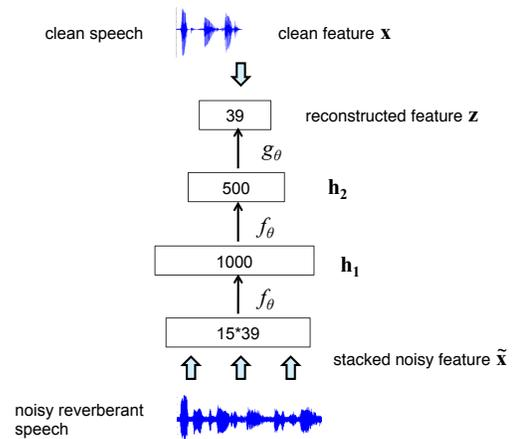
**Fig. 1.** Deep Denoising Autoencoder Architecture. This figure gives an example of a DDA containing two encoder layers, with 1000 nodes and 500 nodes respectively.
