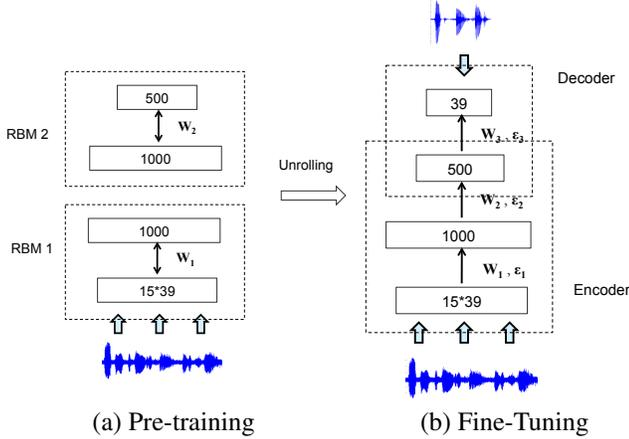
**Fig. 2.** Pre-training consists of learning a stack of restricted Boltzmann machines (RBMs). After pre-training, the RBMs are unrolled to create a deep autoencoder, which is then fine-tuned using back-propagation of error derivatives.
